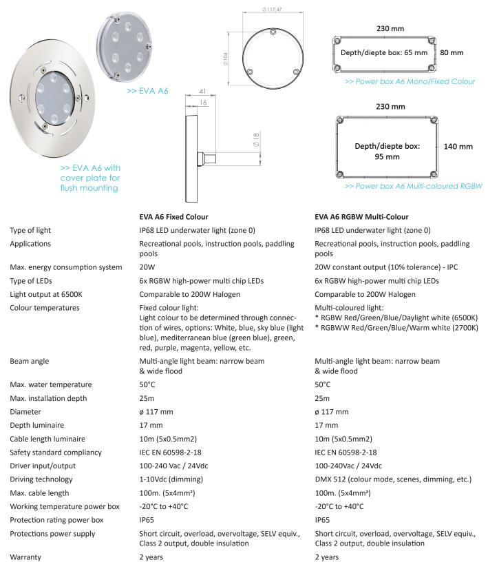
\* Important note! Always provide sufficient space around both luminaire and power box to allow for cooling
